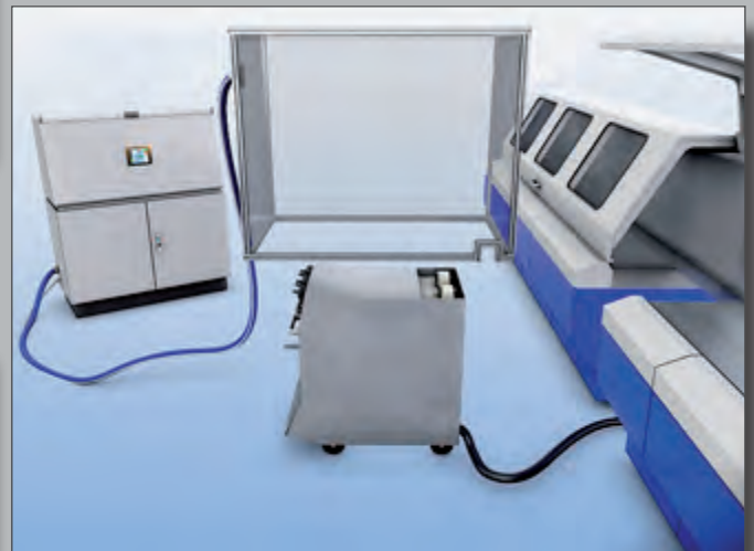
The dry-air box placed over the glue-trolley
