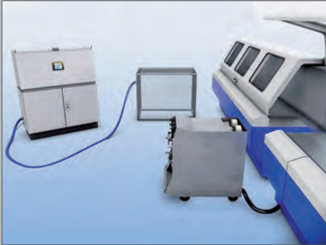
Take out the glue-trolley, not cleaning the system
